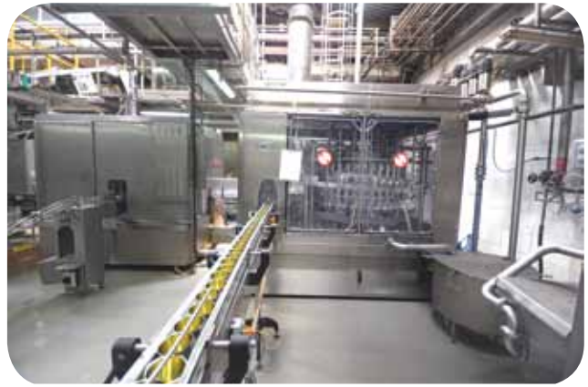
Refurbishment of three (3) old seamers/fillers and the procurement of a new high speed filler will reduce wastage in the milk filling sections of the Evaporated Milk Factory.
